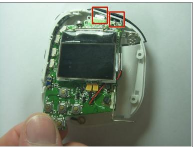
Once those screws are removed, gently remove the board from the rear casing.
