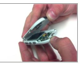
Separate the front housing from the back housing using your thumbs. Carefully pry around the edge of the bottom of device then be sure to unhook the clip inside just below the hold switch.
