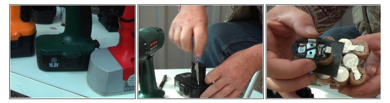
This battery operation concerns 12Volt, 14.4V and 16,8V cordless drills. First open the pack. Take out the battery cells. and disconnect the connector on the top.
