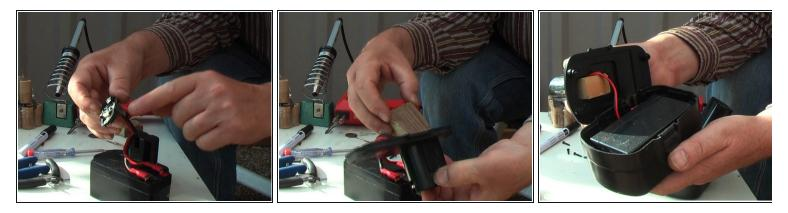
• When the cable is done we can push the top connector back. To hold this in place we have to make a spacer from wood.
