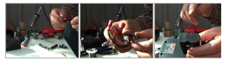
• Next step is to take a 15cm long speaker cable. To one side you press 2 slide connectors. The other side you solder the top connector of the old battery pack. take care with the polarity. You can see the plus and the minus on top.
