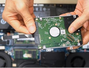
Attach the SATA connector to the HDD.
