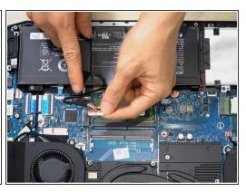
• Unplug the battery cable from the connector attaching the battery to the motherboard.
