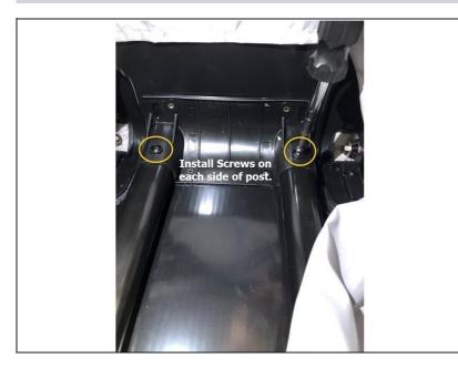
• Once the New Handle is in place, install screws into bottom post. Do not over tighten.
