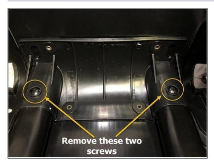
• Locate Bottom Handle Post and remove the 2 screws.
