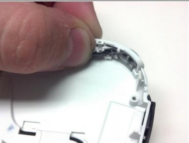
Remove the Volume button from its rocker socket by gently pushing in on the button until it pops out if the two sockets.
