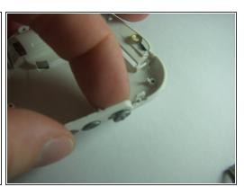
Remove Hold Switch from Socket by squeezing the prongs that hold the button in the socket together and push the button outward.
