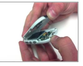
Separate the front housing from the back housing using your thumbs. Carefully pry around the edge of the bottom of device then be sure to unhook the clip inside just below the hold switch.
