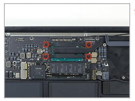
Remove the four 2.5 mm T5 Torx screws securing the heat sink to the logic board.
