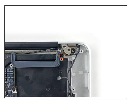
Push the antenna cable retainer out of the way and remove the single 3 mm T5 Torx screw securing the end of the heat sink to the upper case.
