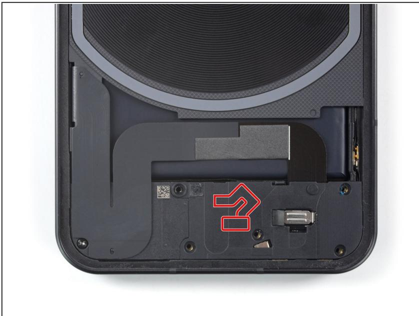
**⚠** When prying up the daughterboard cover in the following step be very careful and avoid levering with too much force or to press your prying tool too deep underneath the cover. Otherwise, the fingerprint cable running underneath can be easily torn.
