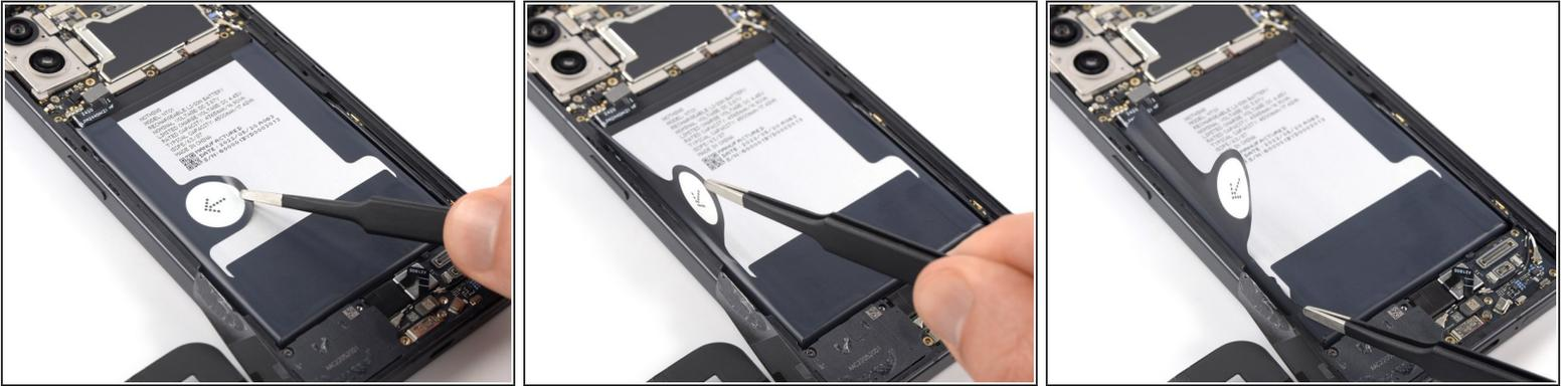
**⚠** Take care not to puncture or bend the battery with your tool—a punctured or bent battery may leak dangerous chemicals or cause fire.
