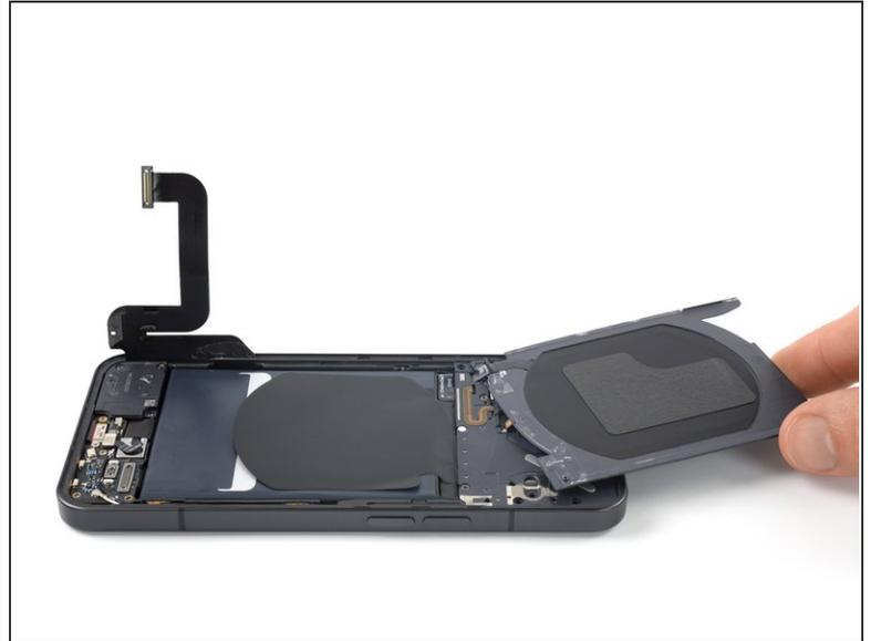
**⚠** When folding the charging coil assembly over avoid straining components and cables.
