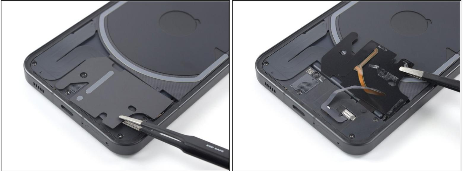
**⚠** The bottom LED assembly is still held in place by a small piece of adhesive sitting between the cable winds. Avoid straining or tearing the cable when folding the assembly over.
