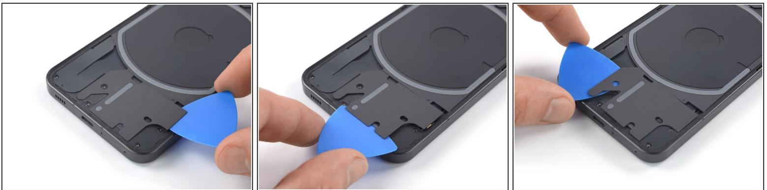
**⚠** Be very careful when working on the bottom LED assembly. There's a [cable running underneath](#) its whole surface that can be damaged easily.
