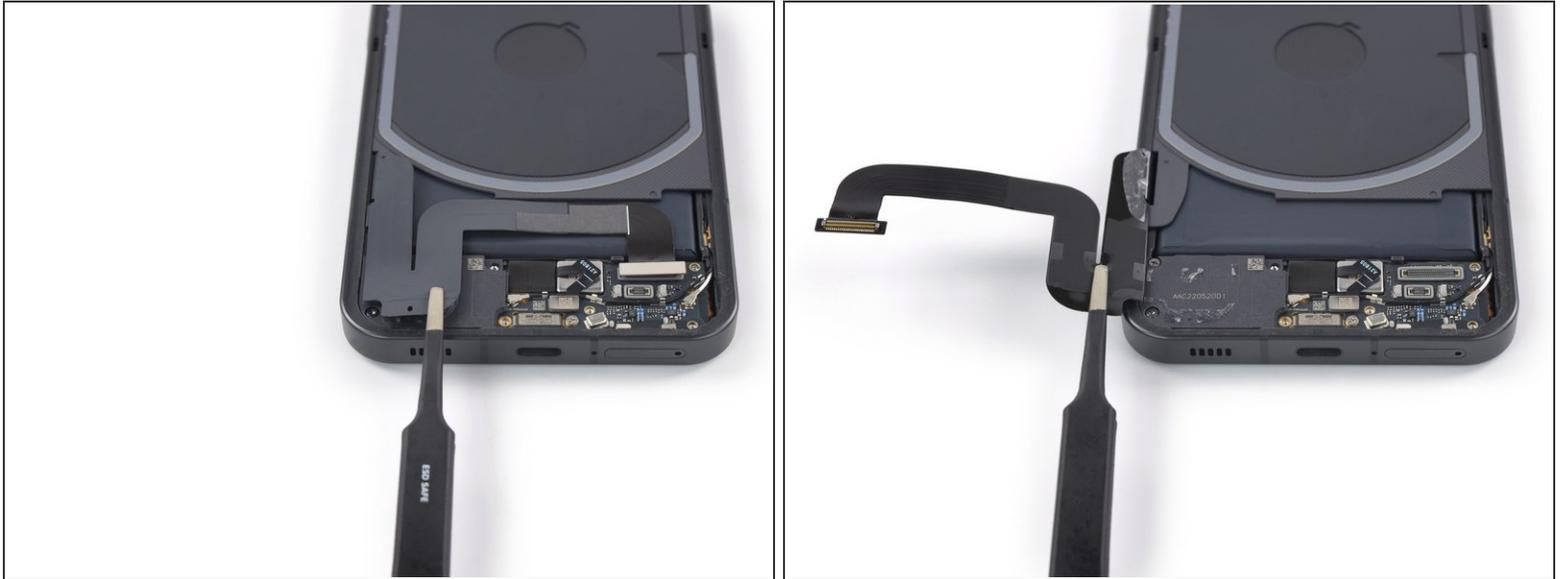
**⚠** During the following step do not fold the cable sharply and only bend it to avoid cable damage.
