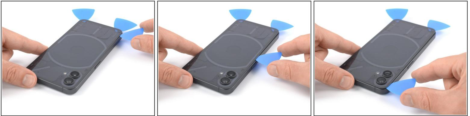
**⚠** When you slice near the glyph, insert only the tip of the opening pick (~2-3 mm) to avoid damaging the LEDs.
