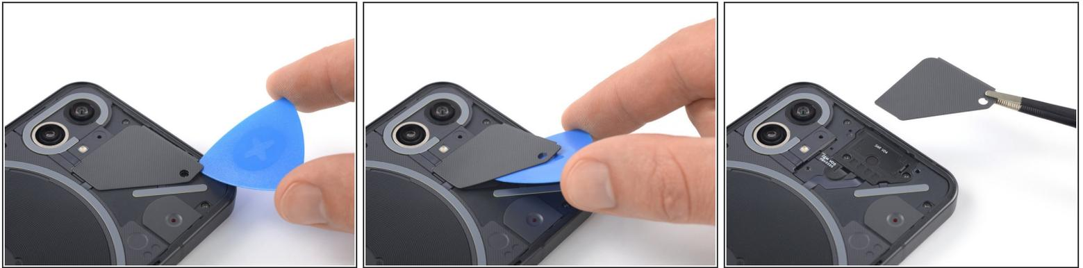
**i** The plastic covering the earpiece speaker is held in place by mild adhesive. If you're having a hard time removing it, apply a [heated iOpener](#) for 1-2 minutes to loosen the adhesive underneath.
