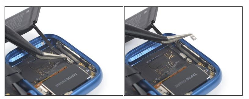
Use a pair of tweezers to remove the battery connector bracket.
