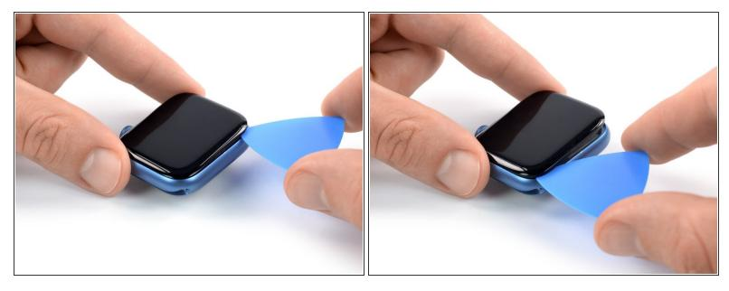
Slide the opening pick around the corner and along the long edge on the opposite side of the watch crown to slice the display adhesive.
