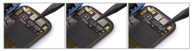
Use a spudger or one arm of your tweezers to pry up the lock bar on the ZIF connectors securing the display cables.
