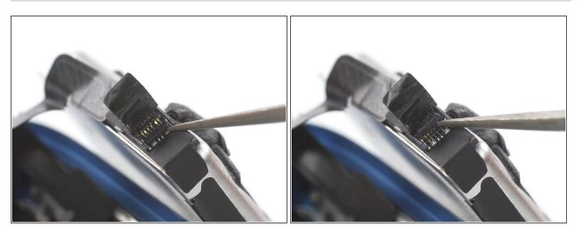
Use one arm of your tweezers or the pointed end of a spudger to pry up the lock bar on the ZIF connector securing the battery cable.
