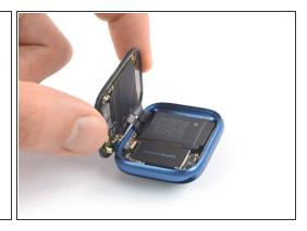
⚠ Be careful not to strain the display cables when you fold the display to the side.
