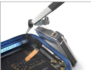
Use a pair of tweezers to pull the battery cable out of the battery ZIF connector.
