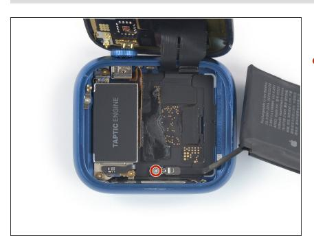
Use a Tri-Point Y000 screwdriver to remove the 1.1 mm-long screw securing the battery connector bracket.
