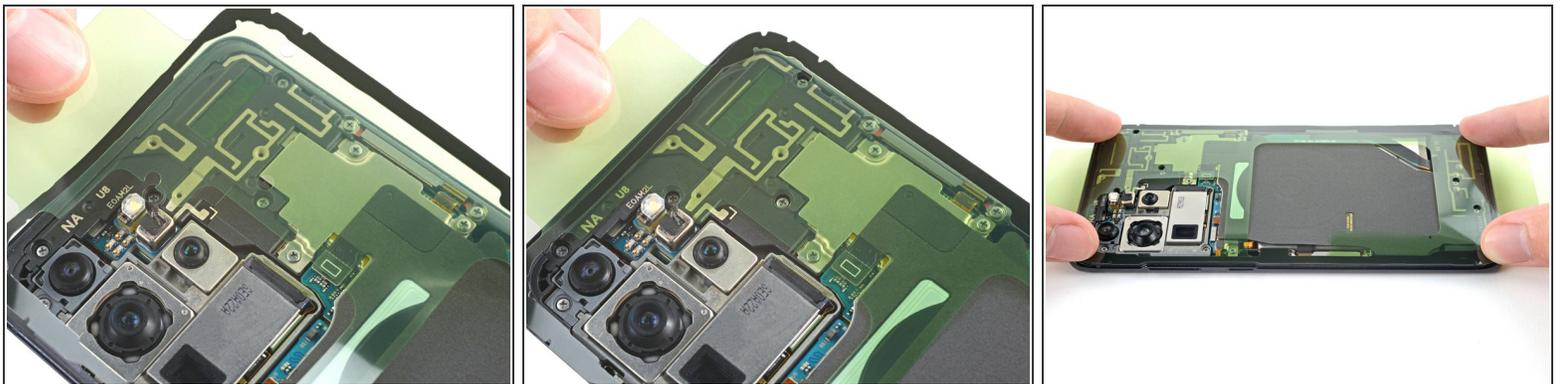
**⚠** Be very careful with this step, as misaligning the adhesive can cause it to peek out of the phone during reassembly, leading to an improper seal.
