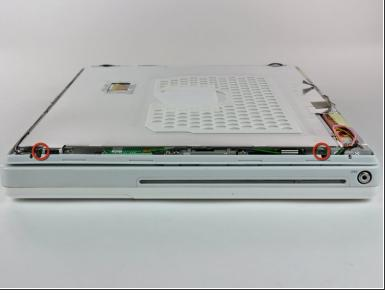
Remove the two Phillips screws securing the left and right sides of the LCD to the frame of the clutch hinges (four screws total).
