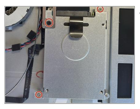
Remove the 3 screws highlighted in red with a <u>000 Screwdriver</u>
