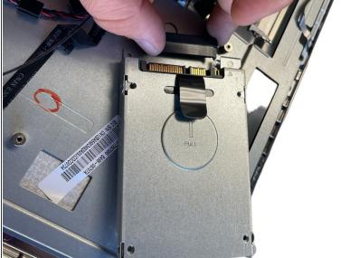
• Once the shroud surrounding the hard drive is free, disconnect the hard drive by grasping the connector with one hand, and the shroud with the other hand and gently pull them apart.
