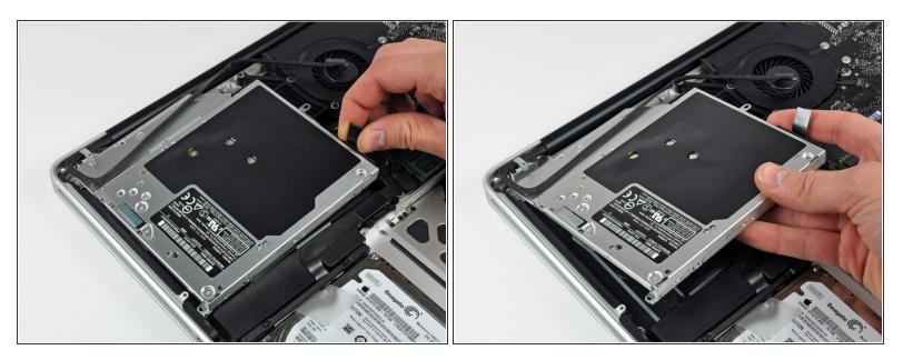
• Lift the optical drive from its left edge and pull it out of the computer.
