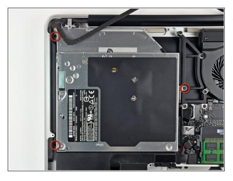
Remove three 3.5 mm Phillips screws securing the optical drive to the upper case.
