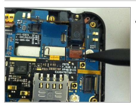
Release the headphone jack's flex cable from its connector
