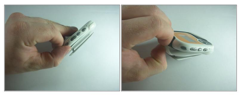
• Remove the belt clip by pulling the clip casing up and away from the device starting at the top over the slightly protruding headphones jack.
