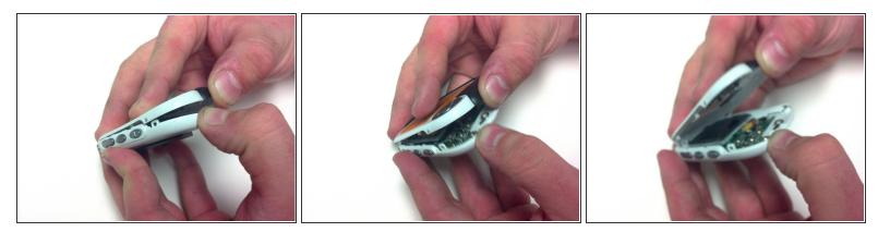
• Separate the front housing from the back housing using your thumbs. Carefully pry around the edge of the bottom of device then be sure to unhook the clip inside just below the hold switch.
