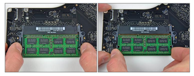
• Release the tabs on each side of the RAM chip by simultaneously pushing each tab away from the chip.
