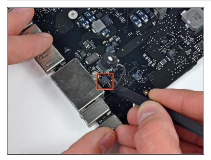
• Use a spudger to pry the microphone cable connector up off the logic board.
