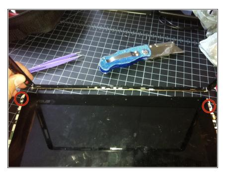
There are four screws to remove behind the bezel. I never got a good picture of the screws but two are indicated here and the other two are in a similar location but just out of the picture.
