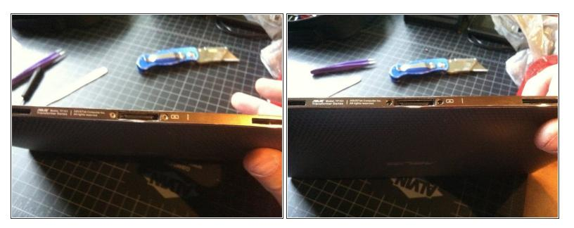
The first step is to remove two Small Torx Screws on the bottom. I don't know the size as I
