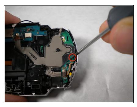
Use a Phillips #00 screwdriver to remove the screw located on the power switch board.
