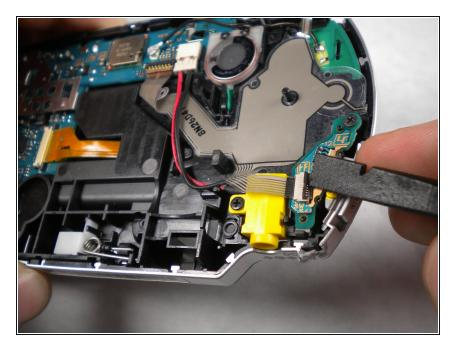
Using a spudger, lift up the lock and remove the ribbon cable from the motherboard
