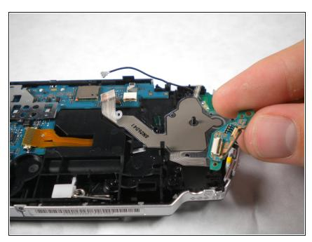
• Lift up and remove the power-switch board.
