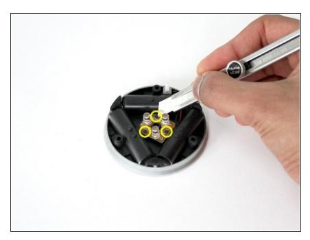
Using the craft knife, slice off the black plastic extrusions at the indicated positions. These tabs secure the circuit board to the main assembly.
