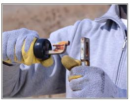
Unhook the first connection by pushing it out and down, then pulling it away from the rest of the rod.
