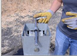
Insert the T-handle into the top cylinder of the exposed pump rod.
