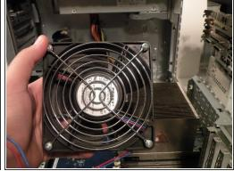
Grab the system fan by its sides and pull it up and out. The system fan is very large and loud, compared to standard sized fans. To reassemble your device, follow these instructions in reverse order.
