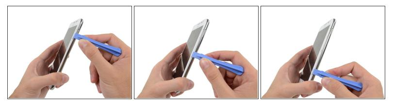
• Slide the plastic opening tool down the seam.
