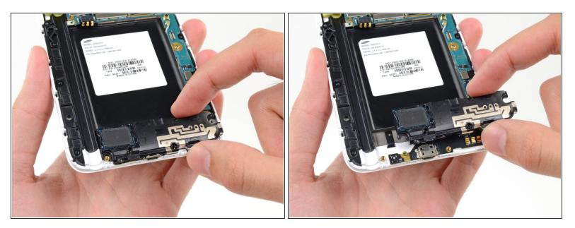
• Remove the speaker enclosure from the display assembly.
