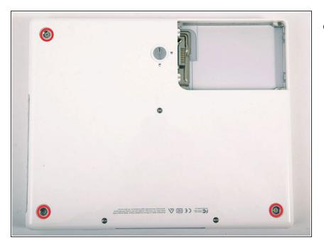
Remove the three newly-revealed Phillips screws.
