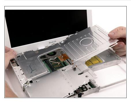
Lift the top shield up from the right side, minding the upper left corner, which may catch on the metal framework. To reassemble your device, follow these instructions in reverse order.
