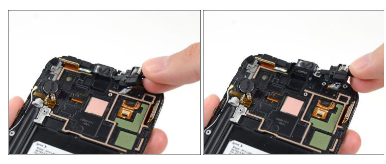
Gently pull the headphone jack straight up without twisting the cable to remove the earpiece speaker portion from its recess.
