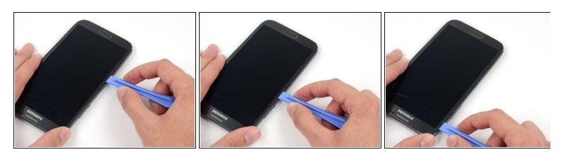
• Continue to run the plastic opening tool down the seam.
