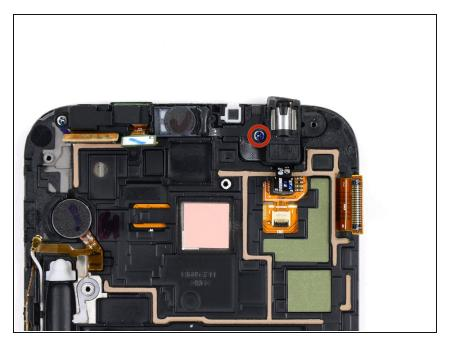
Remove the 3 mm Phillips #00 screw securing the headphone jack assembly to the display assembly.
