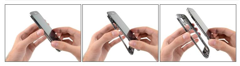
• Remove the midframe from the display assembly.
