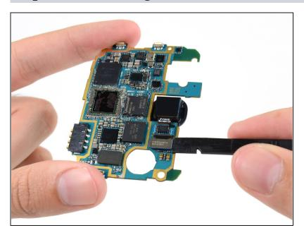
Use the flat end of a spudger to disconnect the rear-facing camera connector.
