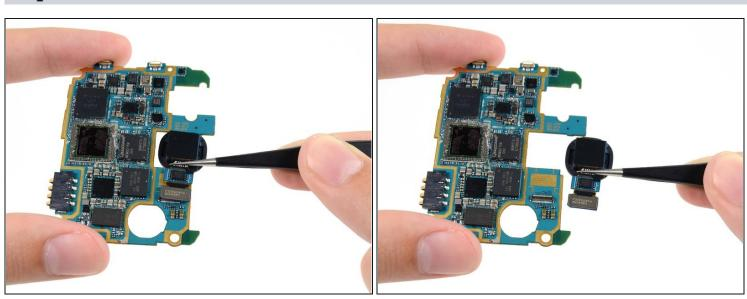
• Using tweezers, or your fingers, slide the rear-facing camera out of its notch in the motherboard.
