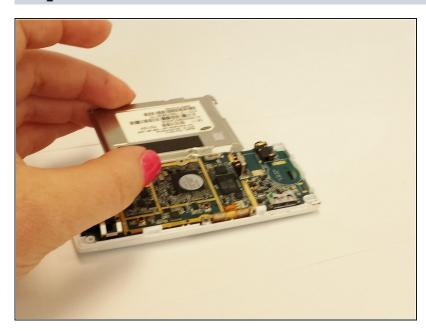
• Lift the metal plate off of the motherboard and set it aside.
