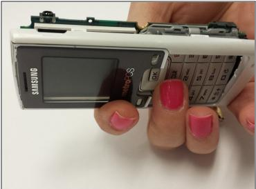
• Push on the white plastic tabs and the keypad at the same time to remove the motherboard.
