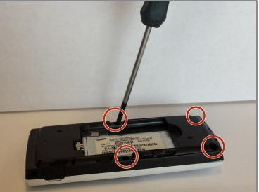
• Remove the four 4.8 mm screws from the midframe using a Phillips #00 screwdriver.
