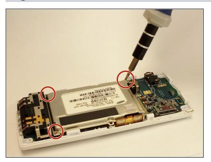
Use a 1.5 mm hex screwdriver to remove the three 2.4 mm screws around the motherboard.
