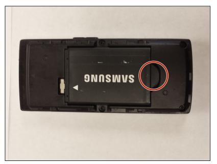
Locate the access notch at the end of the battery compartment.
