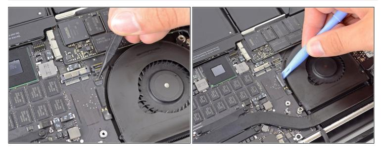
• Use the tip of a spudger to flip up the retaining flap on the right fan ribbon cable <u>ZIF</u> socket.
