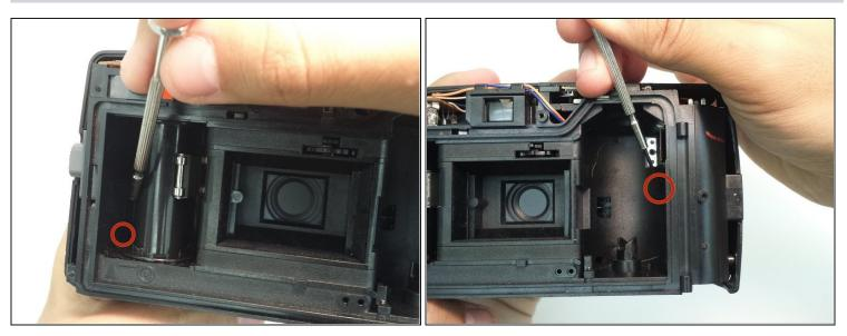
Use a thin shaft screwdriver and unscrew the two indicated screws within the film compartment.
