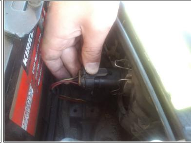
Press firmly on the plugs clip and pull to remove the power cable from the bulb.
