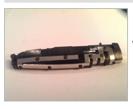
The lower antenna assembly can be similarly removed by applying a little pressure to pop it out of the assembly
