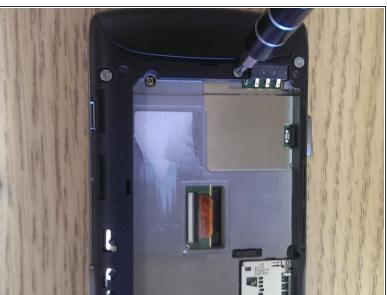
Remove all six screws using a Phillips # 0 (PH0) screwdriver
