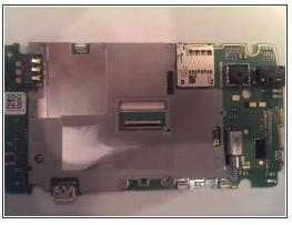
Remove the 3 screws again using the Philips #0 screwdriver. This will allow you to pull out the motherboard from the back housing
