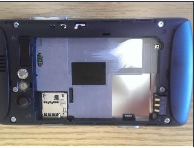
Remove the white sticker to expose the black plastic tab that is covering the ZIF connector that is connecting the flex cable that goes between the motherboard and screen
