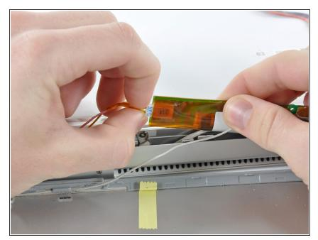
Disconnect the cable by pulling the connector away from the inverter board's socket.
