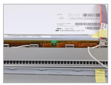
Remove the Phillips screw securing the inverter board.
