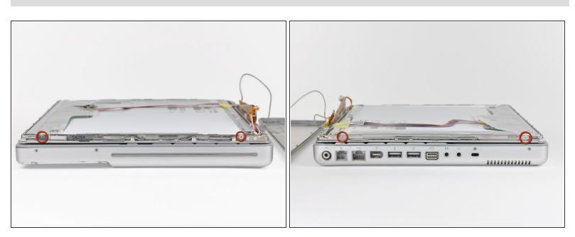
Remove the two Phillips screws from both sides of the display (four in total).
