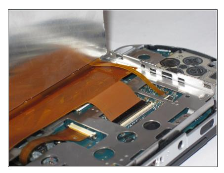
The LCD screen is still attached with ribbon cables. Gently lift up the LCD screen so you do not break them.
