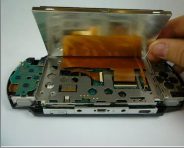
The LCD Screen is held by the LCD Frame with similar clips. Slide a thin tool between the clip and the screen and gently pry them apart while beginning to lift the screen.
