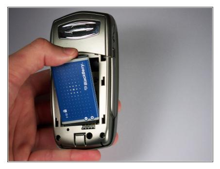
Remove the battery by pushing downward on the area where prongs connect to bottom inside of the phone while using a thumb, finger, or tool to pull on the top of the battery to lift it out.
