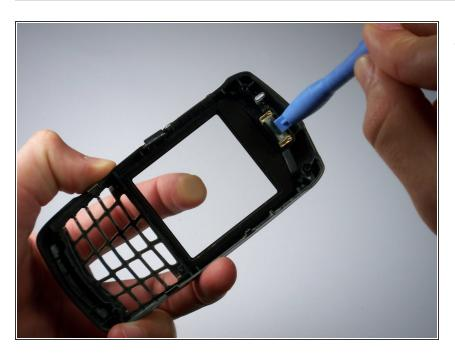
Use the plastic separator tool to apply significant pressure in a downward motion on the top of the white speaker unit.
