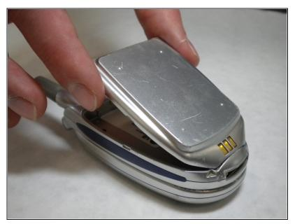
i Remove the battery by lifting up and rotating the battery away from the bottom edge.
