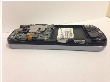
• If the camera button did not fall, carefully remove it using a pair of <u>tweezers</u>. At this point, you can replace the button with a new one.
