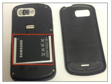
Remove the battery from the phone by pulling up on the battery edge.
