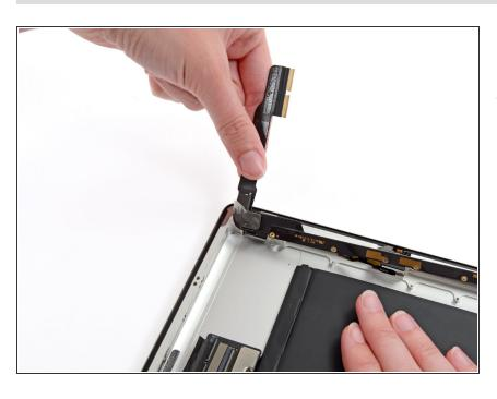
Holding onto the ribbon cable of the headphone jack assembly, carefully pull the assembly upwards towards the top of the device.
