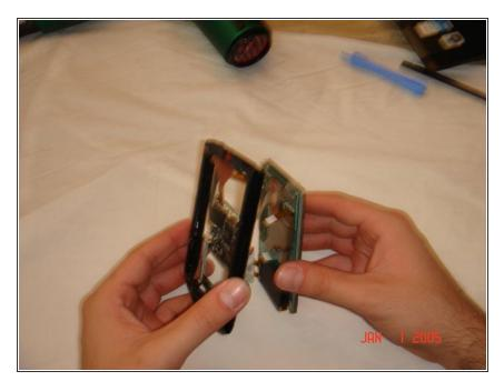
Now that both ribbons and the wire are disconeccted, you can apply a downward pressure to the battery.
