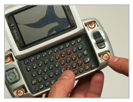
Use the T6 Torx Screwdriver to remove the 4 screws that are underneath the 4 buttons you removed in step one.
