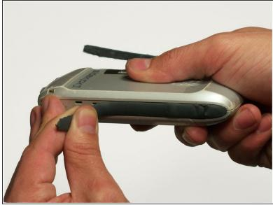
• The bumpers on the top and bottom of the phone can be removed by simply "peeling" them off.
