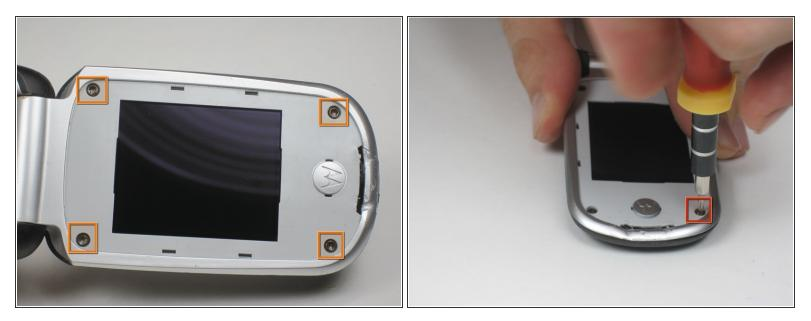
• Unscrew the four screws using the T6 Torx Screwdriver.
