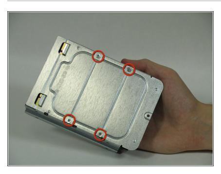
Remove the four screws holding the hard drive to the enclosure.
