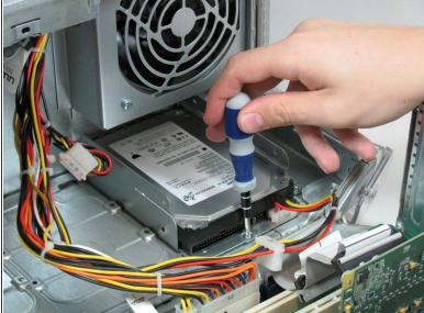
• Remove the screw holding down the hard drive enclosure.
