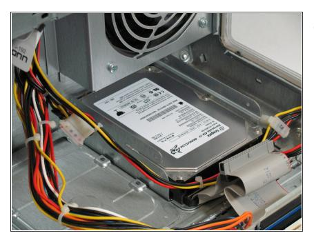
The hard drive is located in the rear right corner of the case.
