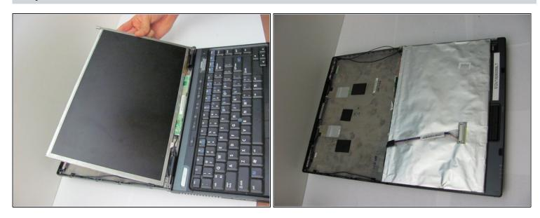
Without lifting the bottom of the monitor, gently flip the screen and lay it face down on the keyboard.
