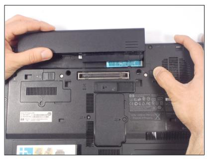
Once both the battery locks are unlocked, slide the battery out to remove.
