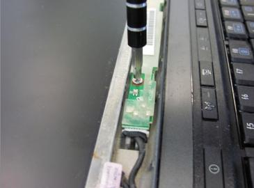
Remove the two 1.2 Philips #1 screws holding down the sensor board at the bottom of the monitor.
