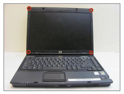
Remove the four 1.2 Philips #1 screws attaching the face plate to the body.
