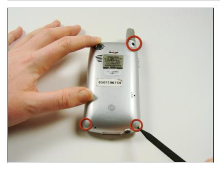
On the back of the device, locate the 3 rubber plugs, and use a plastic spudger to remove them.
