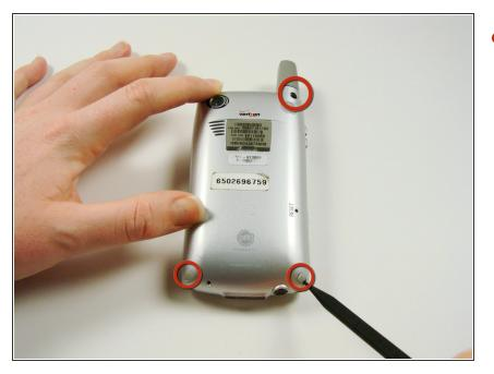
On the back of the device, locate the 3 rubber plugs, and use a plastic spudger to remove them.
