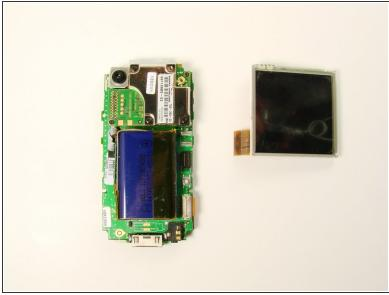
Once the cable is unplugged, you can remove the screen from the body.
