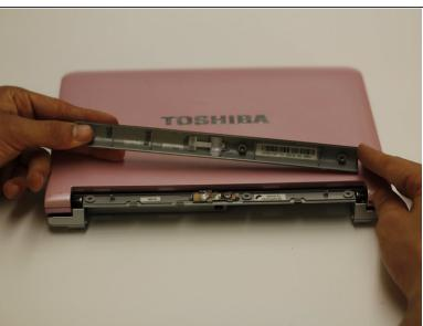
Carefully lift off the power bar assembly for access to the button and receiver.
