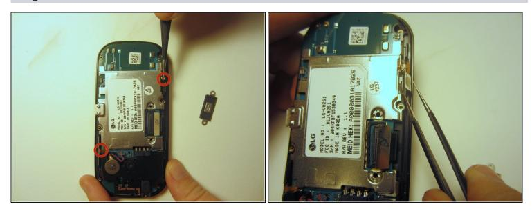
Use <u>tweezers</u> to disconnect the two cables that attach the motherboard to the case.
