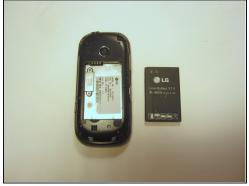
• Use the plastic opener to lift, and remove, the device battery.
