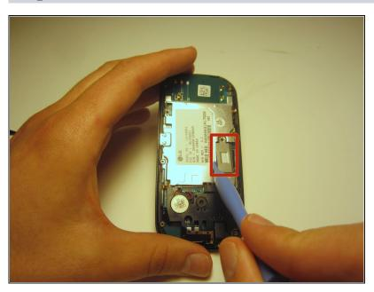
• Rotate the phone 180 degrees and use the plastic opener to lift the metal piece that covers the ribbon cable.
