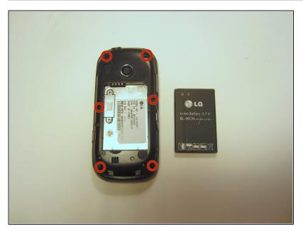
Use a screwdriver and corresponding bit to remove the six 2mm screws that are located along the edge of the rear case. Set the screws aside.
