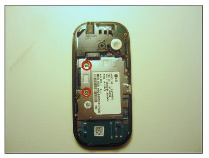
Use a screwdriver and corresponding bit to remove the two 3mm screws that attach the motherboard to the front case. Set the screws aside
