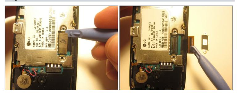
• Use the plastic opener to disconnect the ribbon cable.
