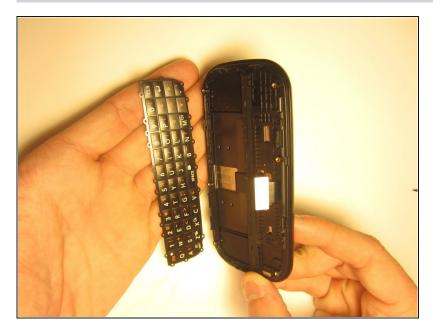
Flip the front case over. If the keyboard doesn't fall out, push it through the front case.
