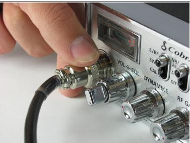
Unscrew the cap counterclockwise on the microphone plug to disconnect the cable.
