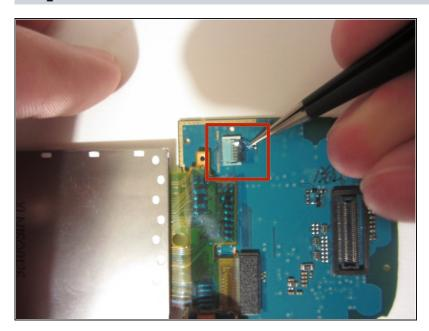
Using a pair of tweezers, remove the tape.
