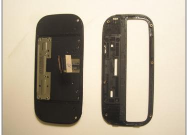
• Pull the ribbon cable through the slit in the keyboard case to separate it from the sliding mechanism.
