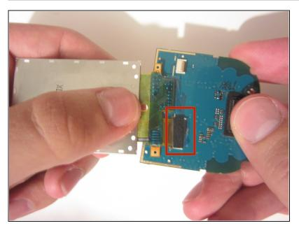
Using either your finger or the plastic opener, disconnect the cable.
