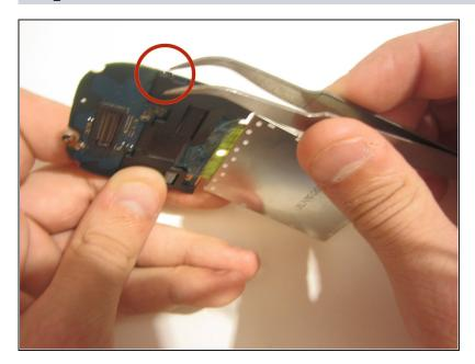
Remove the plastic piece from the circuit board by unlocking the switch on the plastic piece with a pair of tweezers.
