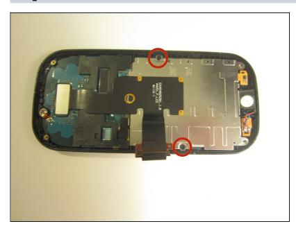
Use a screwdriver and corresponding bit to remove the two 1mm screws. Set the screws aside.
