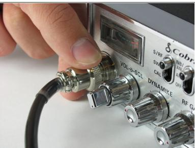
Unscrew the cap counterclockwise on the microphone plug to disconnect the cable.
