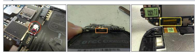
• Now, its time to release the vibrator connector (or vibrator from holder - easier), and then release the lower connector on the main board ( see pic 2). Remove the black tape first, and then use some <u>tweezers</u> to pull out the connector.
