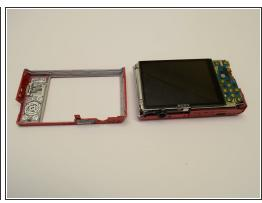
Flip the camera over 180 degrees and similarly pry off the rear casing.
